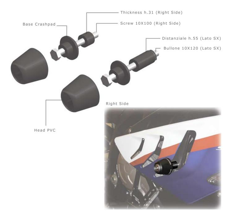
FIND THE FIXING POINT ON THE MOTORBIKE;
