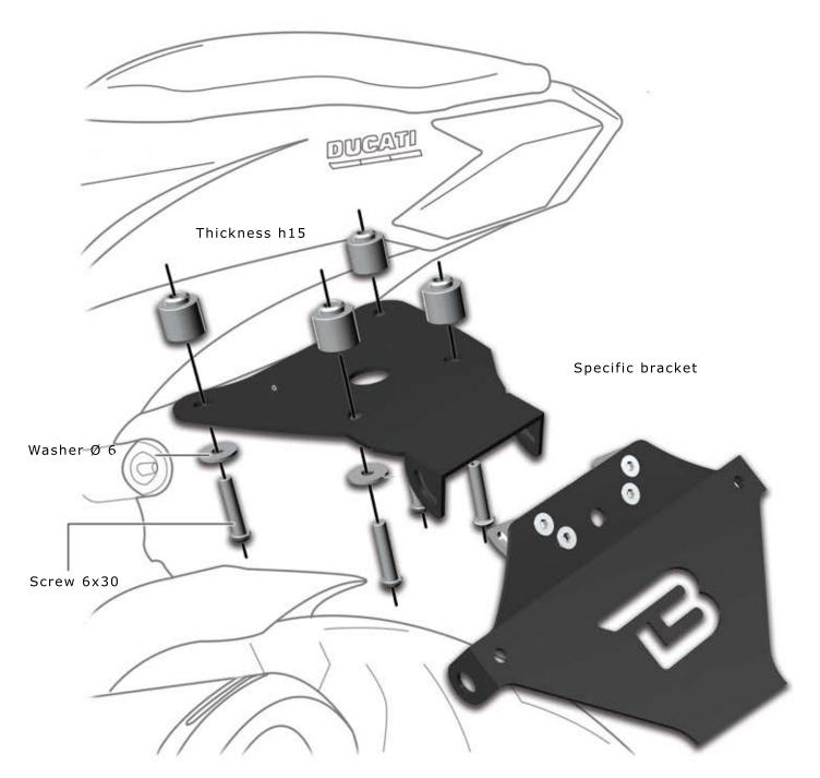
REMOVE THE ORIGINAL LICENCE PLATE. APPLY BARRACUDA LICENCE PLATE FIXING IT WITH ROUND HEAD SCREWS 6X30 LIKE THE PICTURE.
