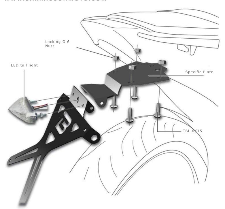
REMOVE THE ORIGINAL LICENCE PLATE FROM MOTORBIKE. APPLY THE BARRACUDA SPECIFIC LICENCE PLATE USING THE TBL SCREWS 6X15 MM INCLUDED INTO THE KIT, TAKE CARE WHILE PASS AWAY THE IN-DICATORS CABLES, TAIL LIGHT AND LED LIGHT CABLES INTO THE SPECIFIC HOLE AND CONNECT THE TAIL LIGHT INCLUDED. FIX ALL LIKE IN THE PICTURE
