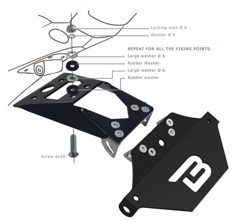
REMOVE THE ORIGINAL LICENCE PLATE. APPLY BARRACUDA LICENCE PLATE BRACKET FIXING IT WITH THE SCREWS INCLUDED (USE WASHERS WITH THE LOCKING NUTS), LIKE THE PICTURE. APPROACH AND LOCK THE LICENCE PLATE TO THE BRACKET JUST INSTALLED.
