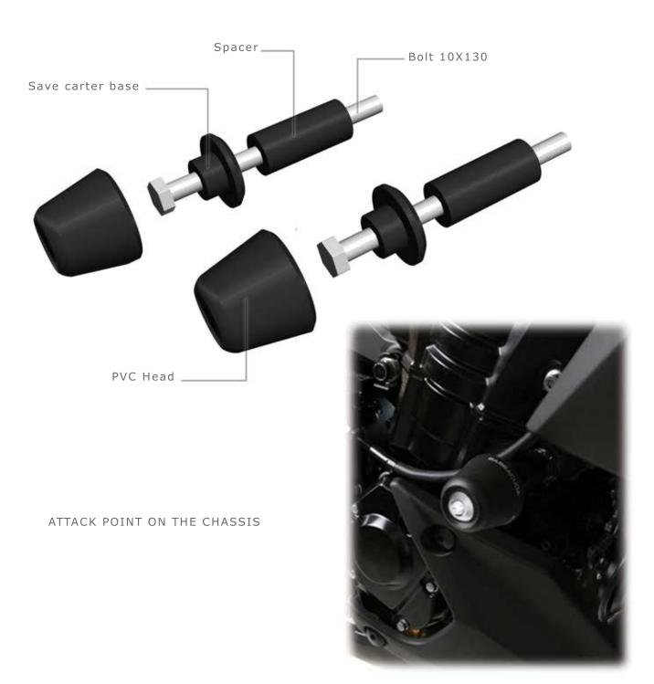
SEARCH AND FIND THE FIXING POINT ON THE MOTORBIKE BEFORE START TO MOUNTAIN, USE THE SPE-CIFIC THICKNESS AND BOLTS LIKE DESCRIBED IN THE PICTURE (SO YOU CAN GET THE RIGHT PROMI-NENCE FROM THE MOTORBIKE).
