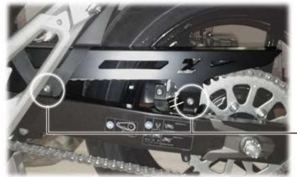
FIX THE BARRACUDA CHAIN COVER WITH THE ORIGINAL SCREWS.
