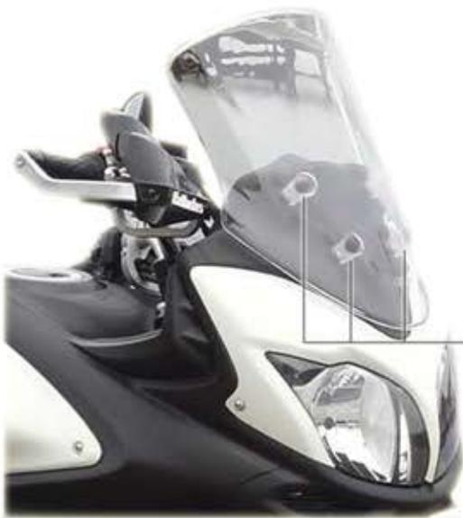
REMOVE THE 4 ORIGINAL FIX SCREWS AND ORIGINAL THICKNESS
