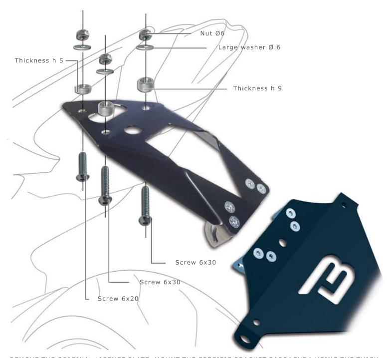
REMOVE THE ORIGINAL LICENCE PLATE. MOUNT THE SPECIFIC BRACKET BARRACUDA USING THE THICK-NESS AND SCREWS INCLUDED INTO THE KIT LIKE SHOWN IN THE PICTURE. USE THE THICKNESS BE-TWEEN THE BRACKET AND THE CHASSIS.
