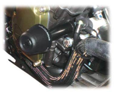
SEARCH AND FIND THE FIXING POINT ON THE MOTORBIKE BEFORE START TO MOUNTAIN, USE THE SPE-CIFIC THICKNESS AND BOLTS LIKE DESCRIBED IN THE PICTURE (SO YOU CAN GET THE RIGHT PROMI-NENCE FROM THE MOTORBIKE).
