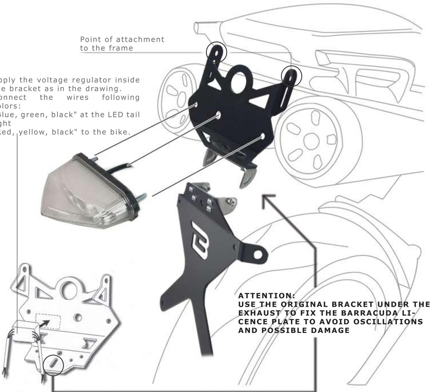
REMOVE THE ORIGINAL LICENCE PLATE. APPLY THE VOLTAGE REGULATOR INSIDE TO THE STRUCTURE OF BARRACUDA LICENCE PLATE (SEE THE PICTURE). FIX THE SPECIFIC BRACKET AT THE ATTACHMENT POINT TO THE FRAME.
