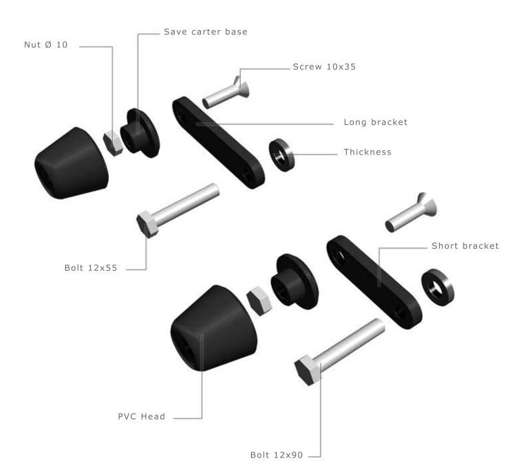
SEARCH AND FIND THE FIXING POINT ON THE MOTORBIKE BEFORE START TO MOUNTAIN, USE THE SPE-CIFIC THICKNESS AND BOLTS LIKE DESCRIBED IN THE PICTURE (SO YOU CAN GET THE RIGHT PROMI-NENCE FROM THE MOTORBIKE). FIX THE PVC HEAD AFTER FIXED AND TIGHTEN ALL THE KIT ONLY
