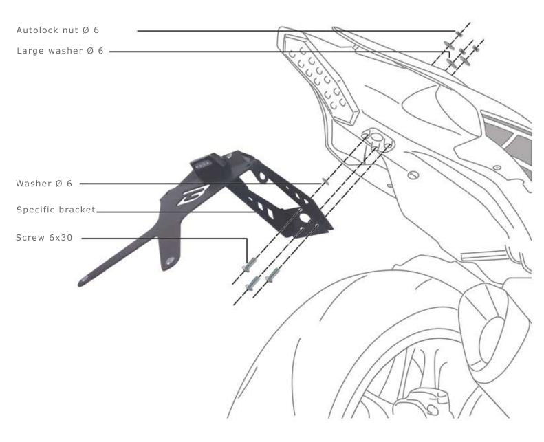
NOTE: WE ADVICE TO TAKE AN INCLINATION NOT EXCEEDING 30° TO AVOID STRUCTURAL POSSIBLE BROKEN
