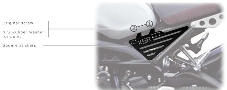
PUT THE SQUARE STICKERS IN THE HIGHLIGHTENED POINTS BEHIND THE BARRACUDA SIDE COVER AND REMOVE THE ORIGINAL SCREWS TO THE POINTS (1) AND (2);
